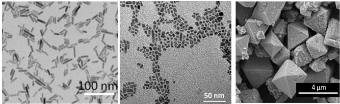
Figure 1. SEM image of ZnO NPs.
