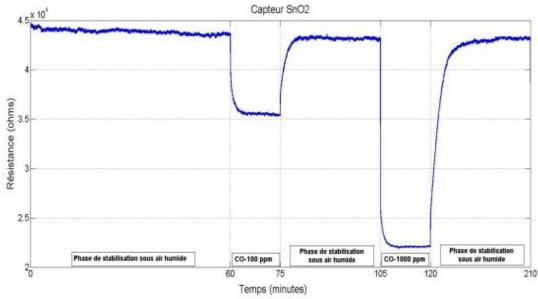
Figure 3. Responses of SnO2 gas sensor at 500°C
