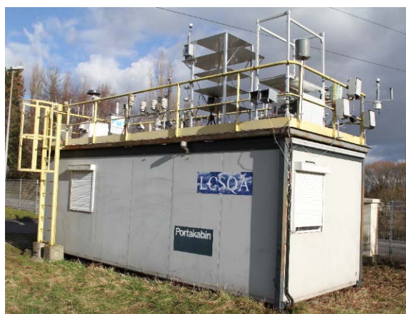
Figure 1 : monitoring station where the sensors systems were mounted.
